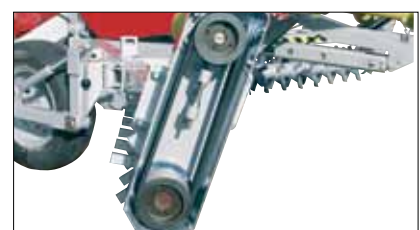
A V-belt pulley powers the stone rakes.
