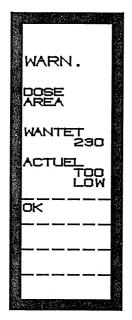
NB: Be aware that sowing shaft electric motor is stopped when the alarm picture is shown.
