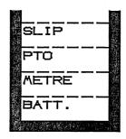
SLIP = Wheel slip PTO = Revolutions on PTO shaft
