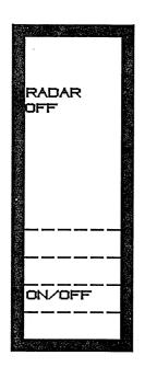
If you wish to use radar (if radar mounted) put radar "ON". At repeated pressure on RADAR ON/OFF you shift between on and off.
