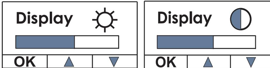
Use the arrow keys “up-down” select, by means of a bar chart, the corresponding value of the brightness of the display. Pressing the “MENU OK” approve the selected level.
