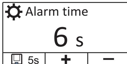
The shorter the response time of the system, the faster we can detect any problems during operation, e.g. locked sowing shaft, low seed in the hopper and so on.
