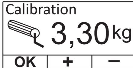
**STEP 5** Weighing the sample of sowing material and check value of seed per hectare.
