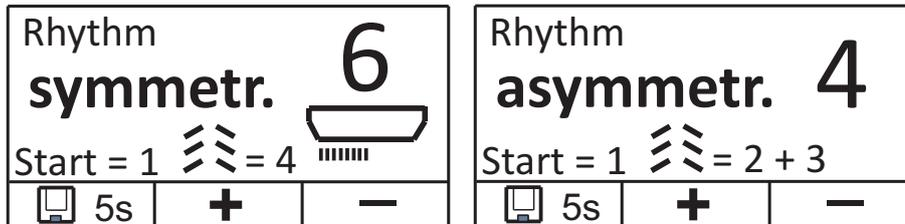
An important principle is that, after setting and approval of all parameters, to start work by pressing the “**WORK**” and setting the markers in the starting position - vertically. Tramlining system is based on counting the movement marks on the headlands (lifting, lowering). The number of the current passage is visible on the screen. When a number is highlighted in black - is made for pass track.
