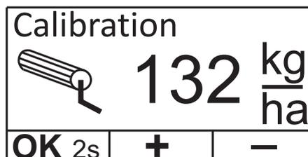
Use “up-down” keys to select the correct numbers on screen and next use “**MENU OK**”. Then time pressing - 2 sec.
