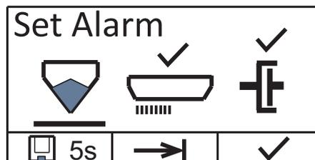
Use the “up-down” select the type of alarm - horizontal bar under the selected icon, and further put a check mark - “bird” - up button. Confirm the settings by pressing the function key “MENU OK” - hold it for 5 seconds. Beep saves the settings.
