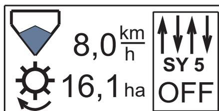
We will see on the screen “**OFF**” This is information that the tramlining system is frozen. At this time it is possible to lower or raise markers without changing the tramline modus. Pressing the “**WORK**” restores the previous settings.
