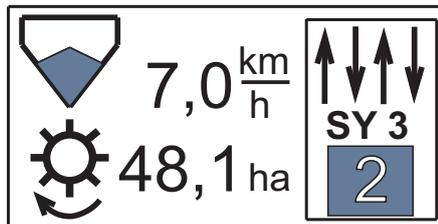
When we choose a tramlining system that requires start work with half the drill, we must equip the drill in the LINAK actuator system. It allows disconnecting the sowing shaft from system level - is not required manually using the “**half width**”
