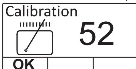
It is recommended to move the lever to a new position according to the value visible on the screen and perform the sowing test again to obtain the expected value of seed per hectare.
