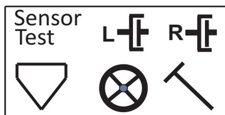
The top row of icons is a state of coupling the left and right control tramlines. The bottom row of icons indicates the level of seed in the tank, turns the sowing shaft and position markers. Covering the sensor in the transmission, e.g. Hand, appears to us a symbol of a full box. By turning the crank sowing shaft - appears to us arrow icon on the wheel, leaving the marks we see the variable position of the marker icon.
