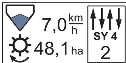
The top row from left: symbol hopper shows us the status of full box of seed (only two states: empty, full), the current speed of the machine and the selected tramlining system.
