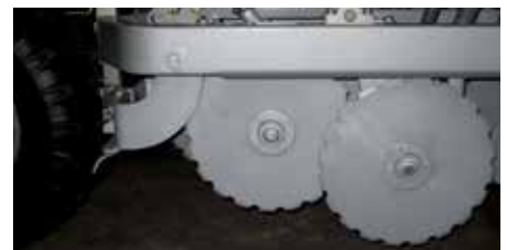
Fertilizer coultters can be raised independently (combi version).
