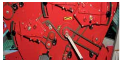
All adjustments on the same side for easy calibration.
