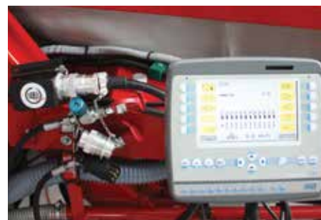
ISOBUS connection and the standard Field-Operator 300 terminal.
