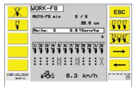
Tramline menu – rows 5 and 8 have been switched off by the automatic tramline controller with row 12 permanently switched off (by the operator).
