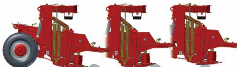
If the cutter bar hits a stone, the top spring is automatically compressed and the machine is lifted so that it can move undamaged over the obstacle.
