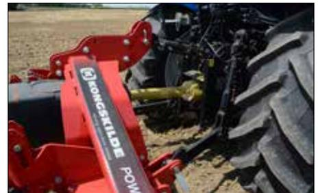
Topmast with integrated bracing.
