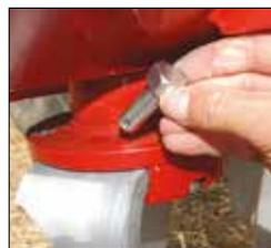
Pin with semi hexagonal head which cannot turn.
