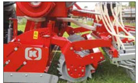
Parallelogram geometry of coultter section coupling. It is not necessary to adjust coultter section position when changing working depth.
