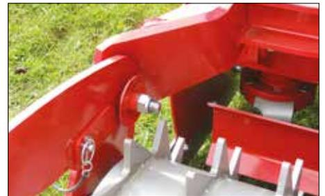
Quick coupling of coultter module on rear roller.
