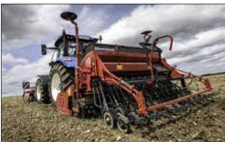
Heavy duty hydraulic combi hitch with MASTERLINE seed drill.
