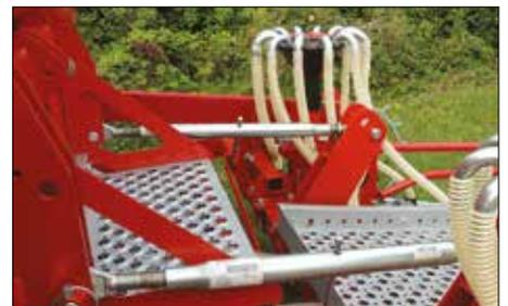
Top connection between coultter section and tank with adjustable top link, allowing level adjustment of coultter module,
