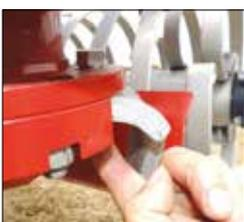
Removal of tine retaining pin which secures the tine
