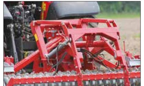
Heavy duty hydraulic combi hitch 3.5 tons lifting capacity.
