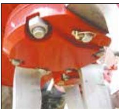
Rubig pin integrated in lower rotor flange.
