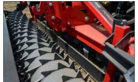
Rear leveling bar fitted on roller arm.
