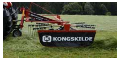
Rake R+ 365 with adjustable swath curtain.
