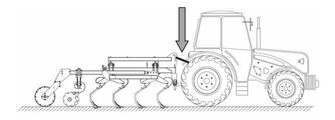
The top link must never be horizontal or parallel to the lower linkages as the cultivator will run unsteadily and make the steering of the tractor difficult.
