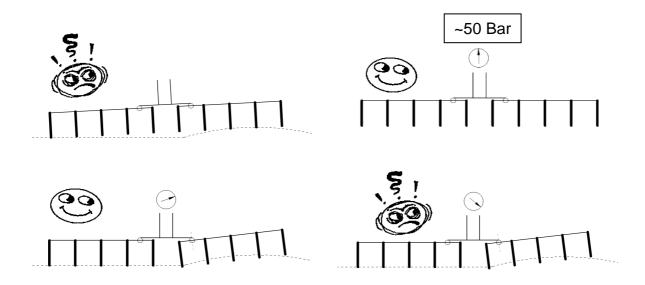
Setting the accumulator pressure is done by pulling the tractors hydraulic lever that is used to unfold Vibro Flex 7400. When unfolded, the value on the pressure gauge will increase. Setting a value of about 60 bar should result in the correct 50 bars when working in the field.
