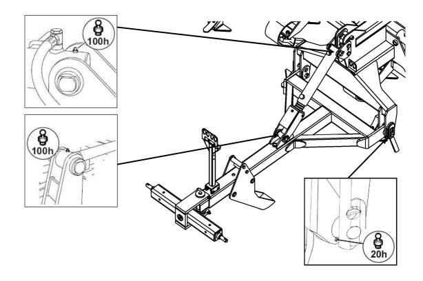
Additional lubrication of front discs (Optional equipment)
