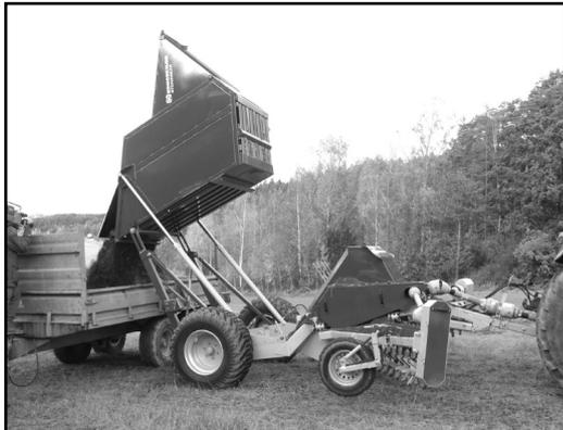
The Stonebear tank will be emptied from the rear by tipping into a trailer or directly onto a tip near the field. When emptying into a trailer, ensure that there is not too much strain placed on the trailer by a sudden or heavy load.
