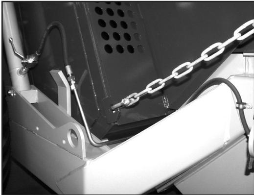
The rakes are lowered into their working position with cables attached to the front of the tank. When lowering the rakes, the lift cables must be attached to the tank mounting brackets.
