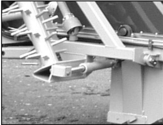
Hydraulic rake lifts are available as optional equipment on the Stonebear. These can also be installed after the delivery of machine.
