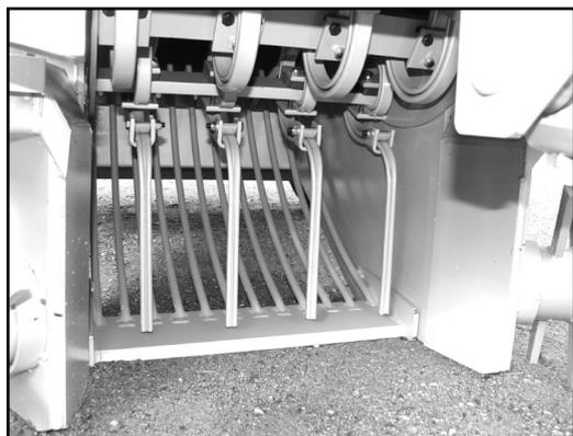
The 40 mm screen is most often included as standard equipment on the Stonebear, as it is well suited to a wide variety of conditions. When clearing land and on grain fields, a screen with 50 mm bar spacing can be used. For replanting lawns and on beet fields, a 40 mm screen is ideal. The tightest bar spacing of the 28 or 35 mm screens are primarily used for potato crops, basic parkland maintenance, and on road construction sites.
