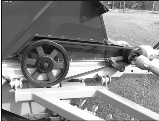
C-belts (2 pcs) transfer the rotation from the gear box to the collecting drum via the auxiliary shaft and belt pulleys.
