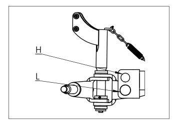
High weight transfer gives better traction, but takes weight off the tractor's front axle. Chose a suitable position considering front axle ballast and the tractor type.
