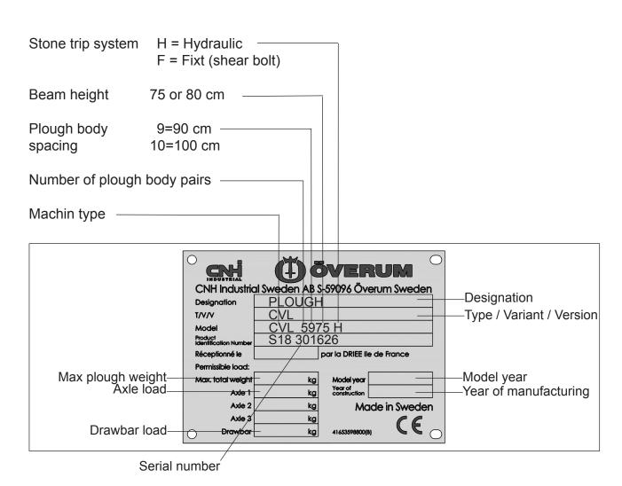
Complete the sign below with the Machine type and Serial number of Your plough.
