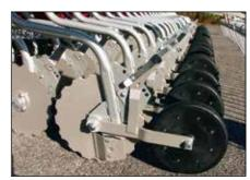
The depth control wheel is very easy and accurately set through a series of holes in steps of 5 mm.
