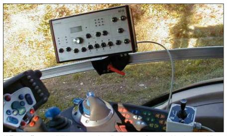
K-Tronic offers possibilities to control application rates from the driver's seat while on the go.
