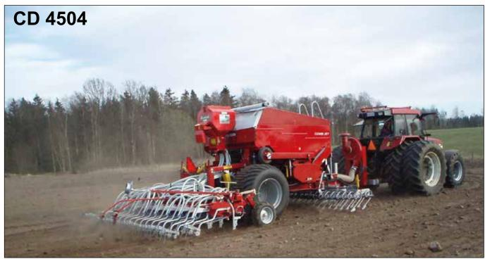
Combi Jet 4504 is built on well proven principals for best possible seed placement. The strong coulter assembly with good clearance together with the possibility to mount the Multi Flex system and full width tyre packers in front of the coulters, give the option to cultivate, reconfirm, fertilise and seed in the same go. The machine above is equipped with optional grass seed box for simultaneous shallow grass establishment.
