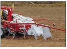
The Multi Jet can be equipped with two rows of harrow tines in the coulter unit, placed to work the soil between each seed coulter.
