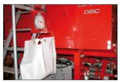
Weighing equipment eases the calibration test
