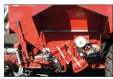
Vario-K gearboxes controlled by K-Tronic offer possibilities to control the application rates while on the go.
