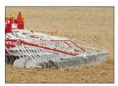
The individually spring loaded scalloped disc coulter on Multi Jet Disc has a pressure wheel consolidating over the seed row. A heavy rear harrow leaves an even loose surface.
