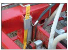
Hydraulic coulter pressure adjustment cylinder with indicator placed on the outer end of the wing section.
