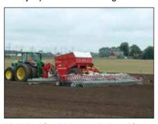
Multi Jet / Combi Jet are designed for a working speed between 10 – 15 km/h.
