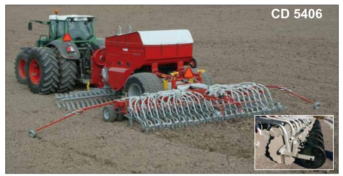
Combi Jet 5406 equipped with Multi Flex system, Full width tyre packer, light following harrow and pre emergence marker, incorporates seedbed preparation, consolidation, fertiliser placement and seeding in one go. All Combi Jet models can also be delivered in disc coulter version for conditions with crop residues.
