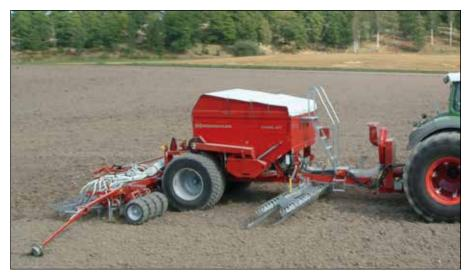
Combi Jet performs seedbed preparation, consolidation, fertilising and drilling in one operation. The Multi Flex system in the front levels, shatters clods and prepare seedbed. The full width packer with tractor treaded rubber tyres crushes and consolidate the seed bed before the narrow fertiliser coulters place the fertiliser underneath the seed depth for optimum combined placement effect.
