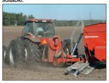
The new cross shaft hitch makes the machine reach the corners and follows the tractor better when turning on the head land.
