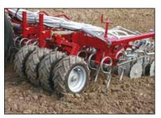
Side packers with two, four or eight threaded rubber wheels can be mounted per side in order to achieve full width consolidation for 4, 6 and 8 m. working width.
