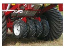
Re-consolidation between the wheels of the tractor can be performed with an accumulator-loaded tyre packer between the large LGP-tyres.
