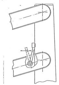
4.8 Always lower the support legs in front of the tool bar when the machine is disengaged from the tractor. Put a pin in each support leg.
