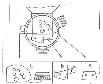
The seed is then caught in an airstream. By means of air as a medium of transport the seed is blown to the furrow.
