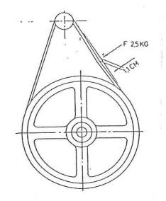
If the belts need tightening, loosen the four bolts securing the blower bracket and tighten the belts with the two tightening screws. Remember to retighten the four bolts that secure the blower bracket.
