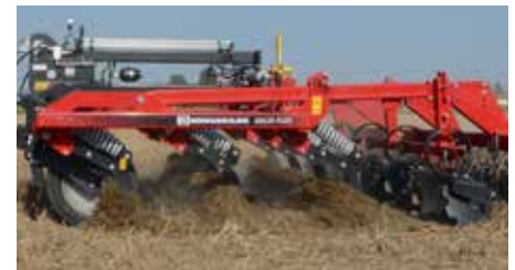
Optimal mixing of soil and residues.
