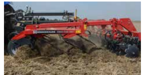
4 rows of tines for a more intensive mixing of soil and field residues.
