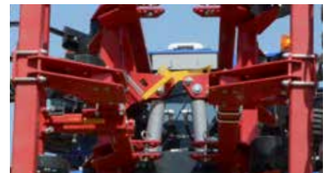
Automatic hydraulic wing lock system.
