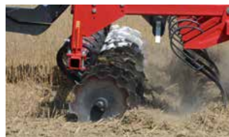
Front disc section - Vibro Flex 7400.
