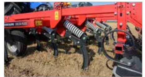
C-shaped Delta Flex tine.
