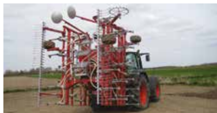
Frame folding in 2 sections ensures 3,0 m transport width.
