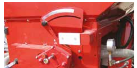
Vario-K stepless transmission.
