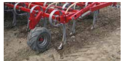
Precise depth control is achieved by the large low flotation tractor pattern tires.
