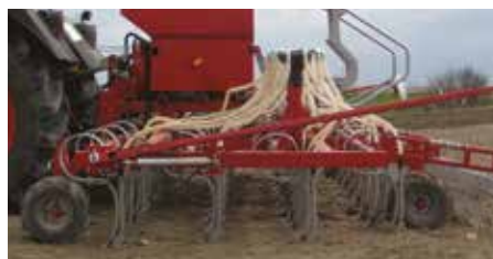
4 rows of tines allows easy passage of field residues.
