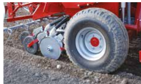
Accurate and reliable metering system driven by large wheels. (optional)
