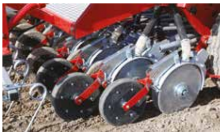
Double disc coulters (DR) with rubber press wheels. (optional)
