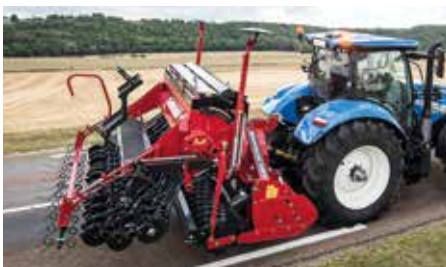
The weight of the drill is carried on the packer roller of the cultivator.
