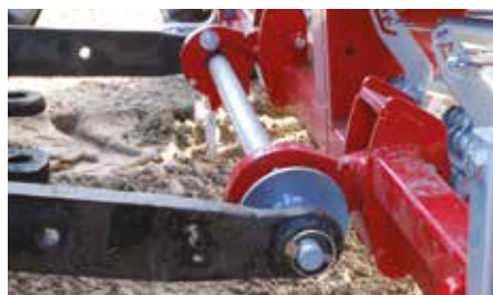
Quick hitch for easy coupling. (optional)
