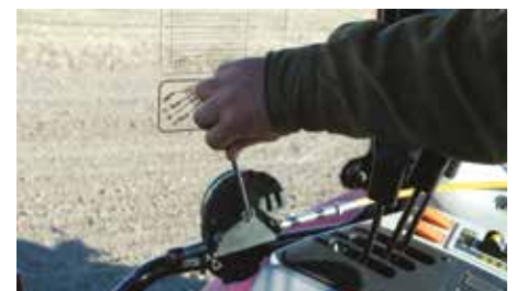
Stepless adjusting of application rate direct from tractor cabin. (optional)
