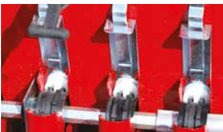
Fine seed fingers for reducing the application rate.
