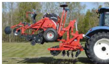
Hydraulic drill linkage for mounting the seed drill on cultivator.
