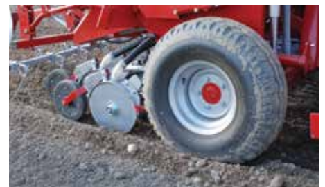
Accurate and reliable metering system driven by large wheels.
