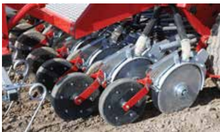
Double disc coulters (DR) with rubber press wheels.
