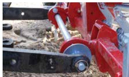
Quick hitch for easy coupling.
