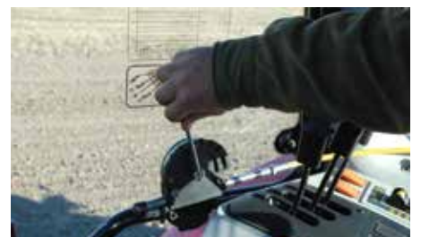
Stepless adjusting of application rate direct from tractor cabin.
