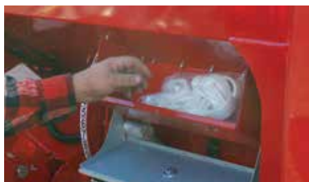
Integrated toolbox for storage of tools, spare parts etc.
