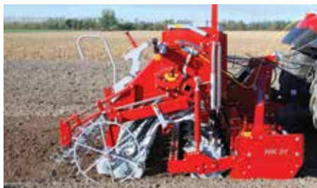
The weight of the drill is carried on the packer roller of the cultivator.
