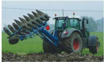
In on-land position the plough is well in balance for turn over.
