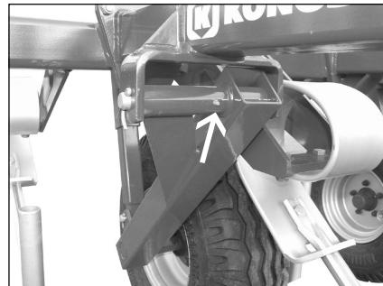
Lubricate wheel hubs and wheel assemblies after every 25 hours of work or at least once a week.
