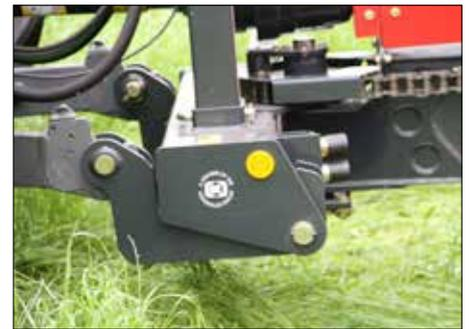
Top safe ensures low impact on the cutter bar while driving with high speed.
