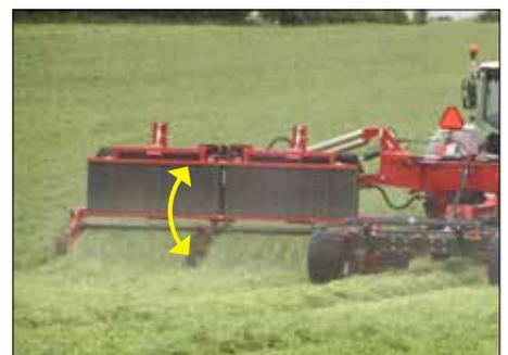
Collector is not activated and the GXT can then make wide spreading.
