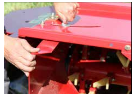
Adjustment of conditioner plate
