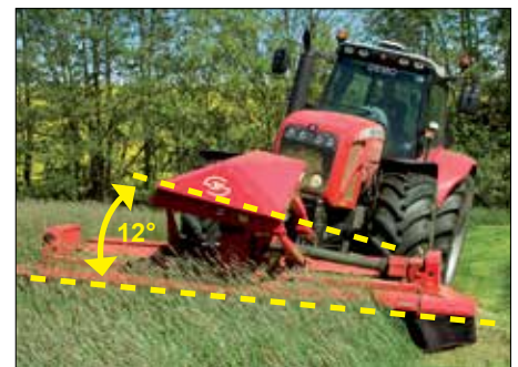
Contour Float - Sideways following
