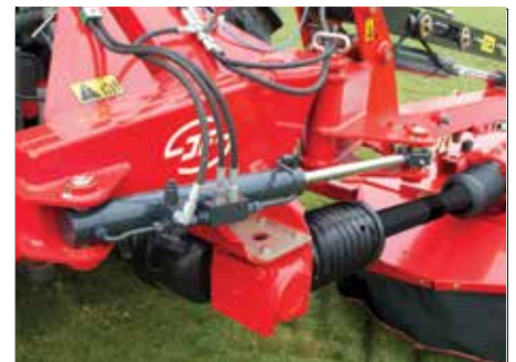
Hydraulic stone release
