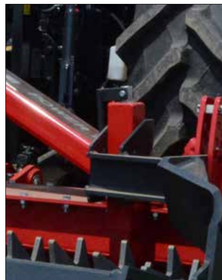
Diepteinstelling via spindel.
