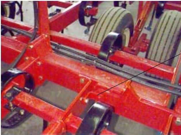
Detail view of frame assembly at front corner showing front hinge.
