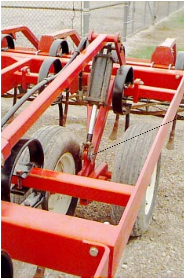
Detail view of tandem wing wheel arm assembly.
