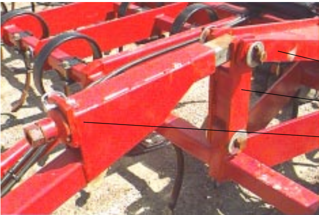
Attach hitch adjuster to the front pivot link with the pin provided.
