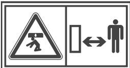
**Make sure that no one is in close proximity of the plough when turnover action is carried out. Never attempt to adjust any of the settings while the plough is in use.**
