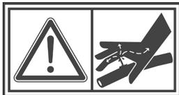
**Never attempt to disconnect any hydraulic connection while the system is pressurized.**
