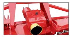
3-speed leverchange gearbox with rear PTO.
