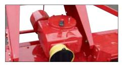
3-speed leverchange gearbox with rear PTO.
