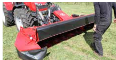
Easy and quick access to the SMF cutter bar.
