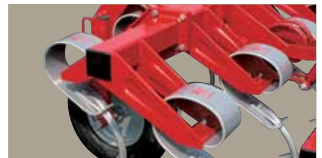
VF 2000 Bolted on side extensions.
