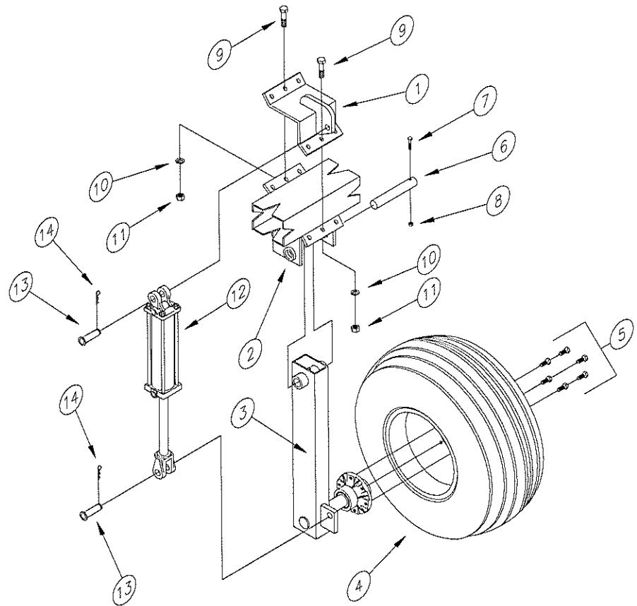
RIGHT OUTER WING WHEEL ASSEMBLY (50' BAR - FEI)
