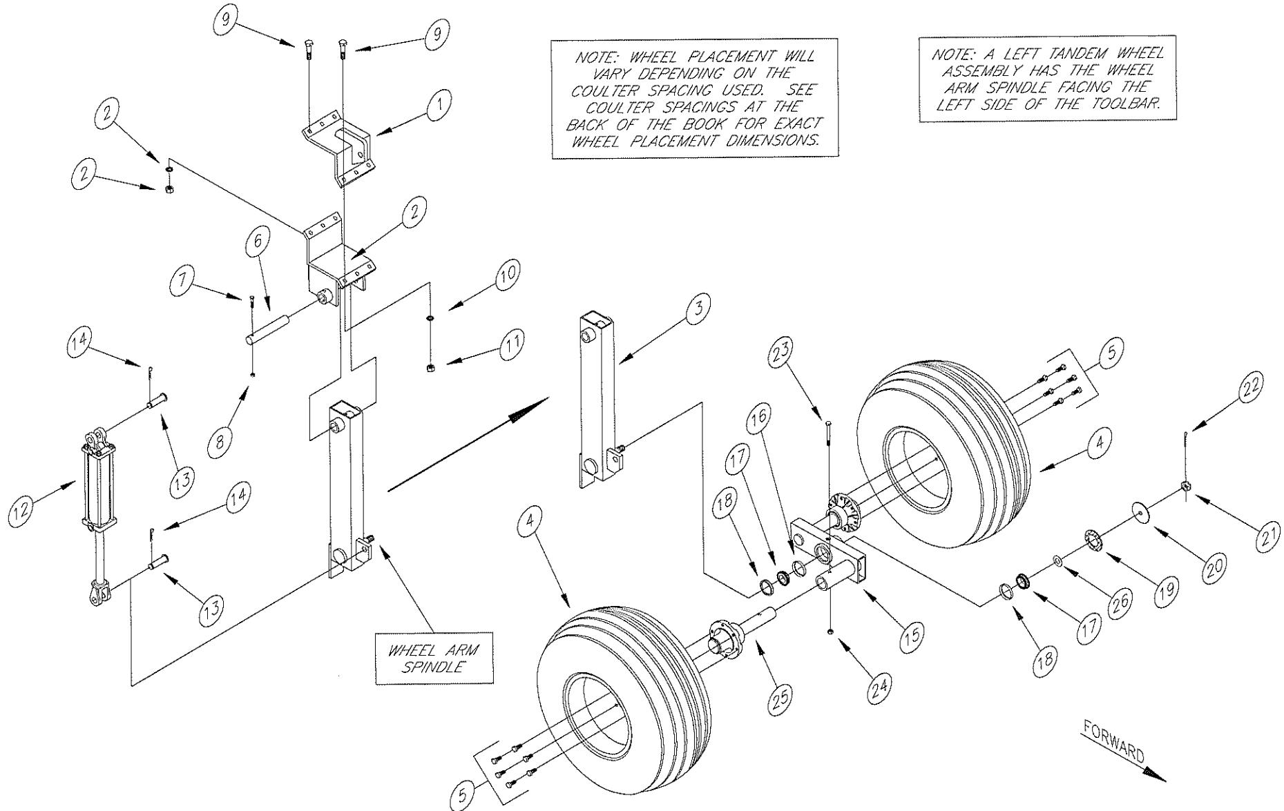
LEFT TANDEM INNER WING WHEEL ASSEMBLY PART NUMBERS (50' BAR - FEI)
