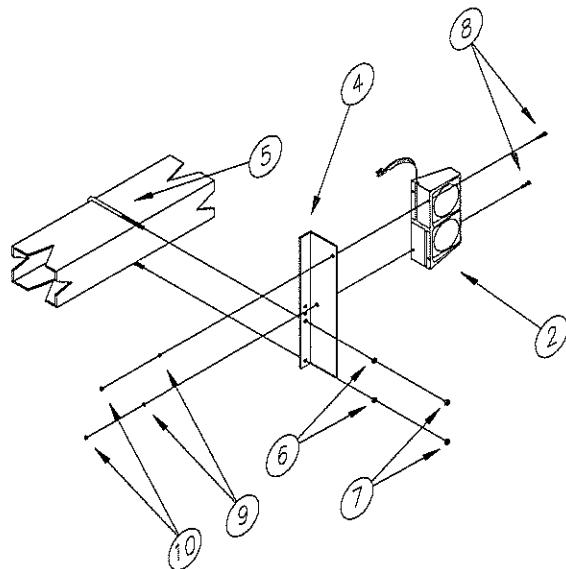
ATTACH LIGHT MOUNTING BRACKETS TO THE REAR TUBE OF THE INNER WING AS CLOSE TO THE MAINFRAME AS COULTER SPACING WILL ALLOW.
