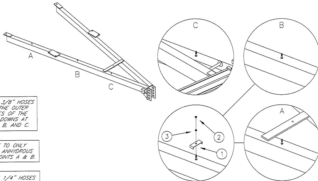
**FASTEN THE 3/8" HOSES TOWARDS THE OUTER EXTREMITIES OF THE HOSE HOLDOWNS AT POINTS A, B, AND C.**
