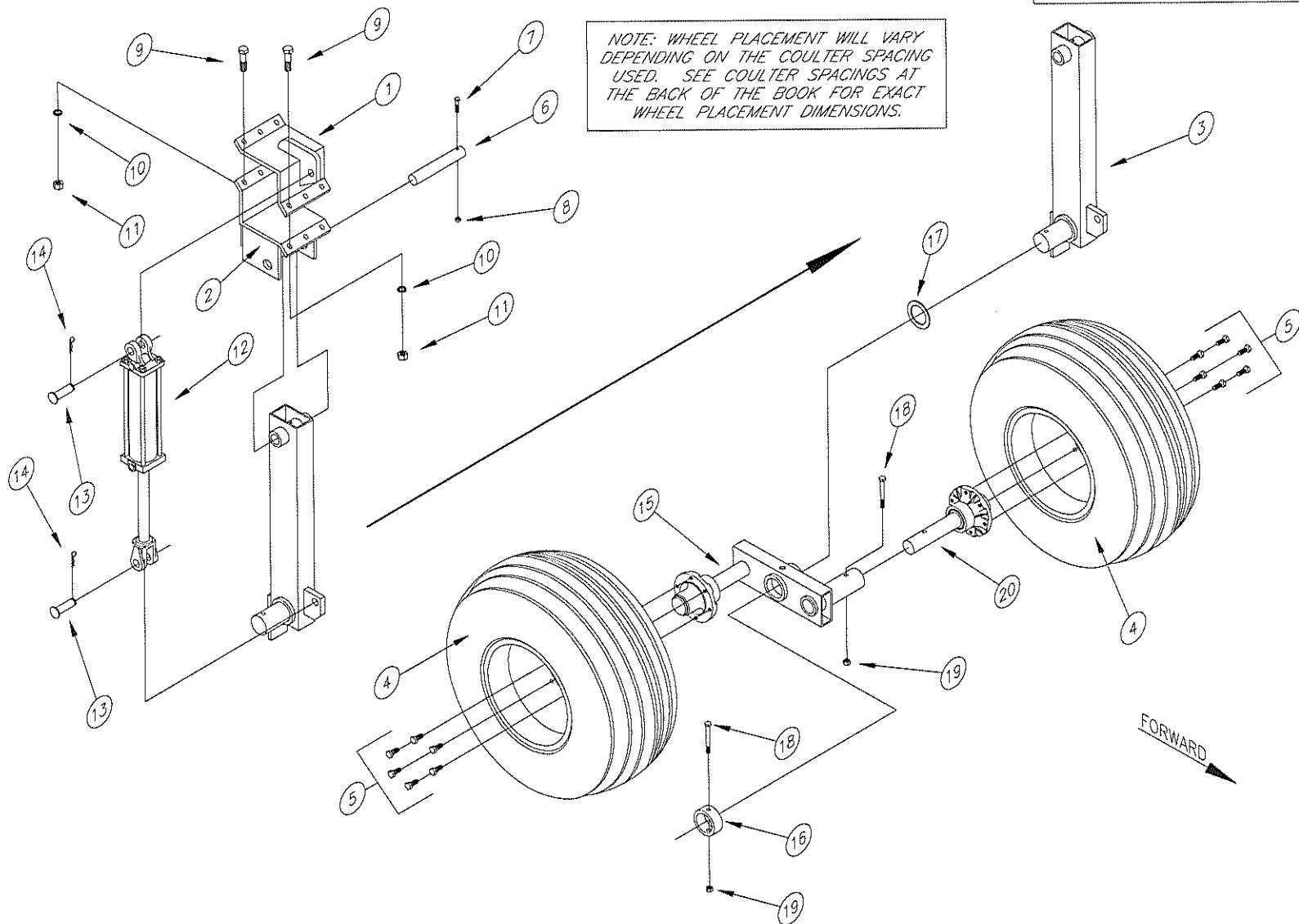
RIGHT TANDEM MAINFRAME WHEEL ASSEMBLY PART NUMBERS (50' BAR - FEI)
