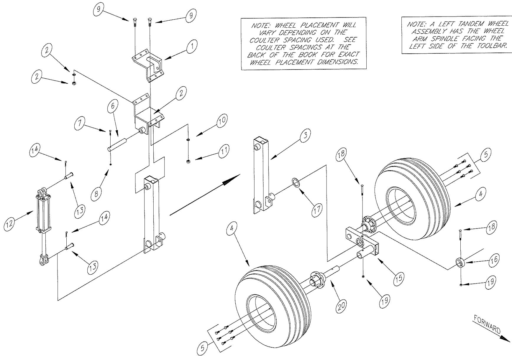
LEFT TANDEM MAINFRAME WHEEL ASSEMBLY PART NUMBERS (50' BAR - FEI)
