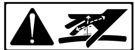
Hydraulic hoses should only be connected to the tractor outlets if the tractor and the machine are pressure-free. If the hydraulics of the tractor is activated it may lead to uncontrolled movements which may cause secondary damage.
