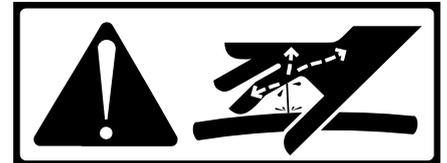
Make sure that no persons are near the machine when starting as there might be air in the hydraulic system which might lead to sudden movements.
