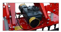
3-speed leverchange gearbox with rear PTO.
