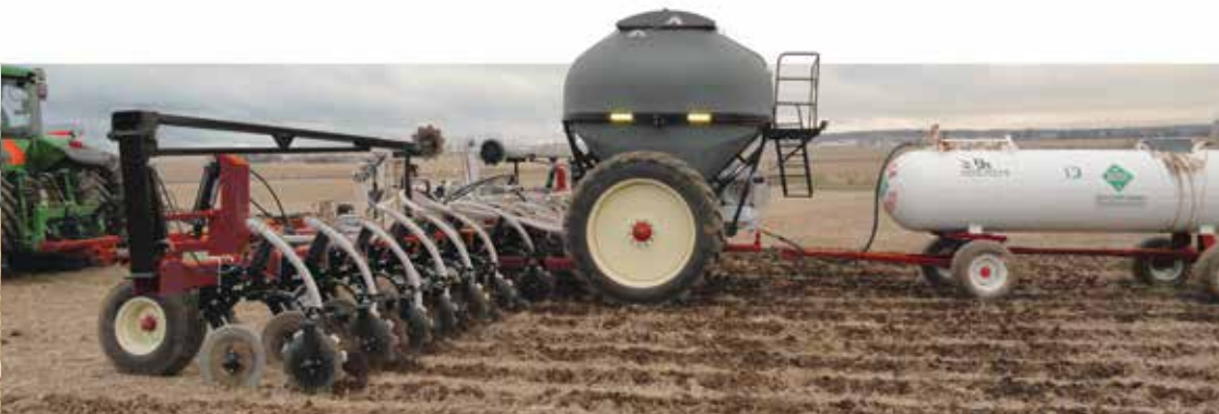
F6200 applying dry and anhydrous fertilizer in one pass
