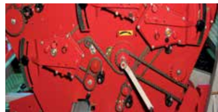
All adjustments on the same side for easy calibration.
