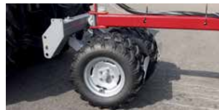
Heavy duty inter wheel packer with 7.50 x 16 wheels (alternative).
