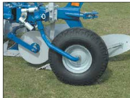
Roue combiné transport/jauge 10.00x12, diam. 710mm, largeur 264mm.
