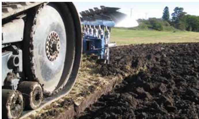
The Vari Flex EX On-land can be hydraulically side shifted to adjust to different tractor widths, and to fine tune the front furrow width.
