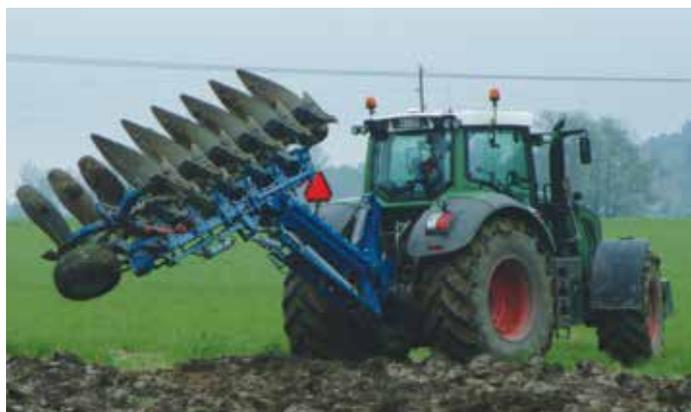
In on-land position the plough is well in balance for turn over.
