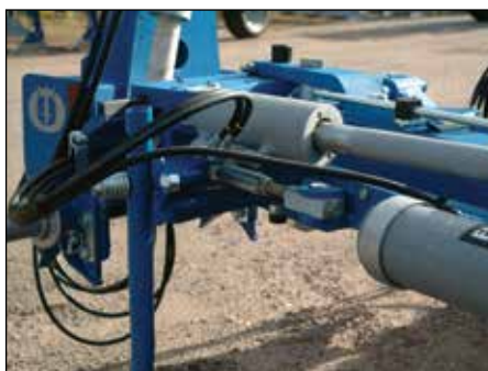
With the turnbuckle all side forces are balanced out for minimum draft requirement.
