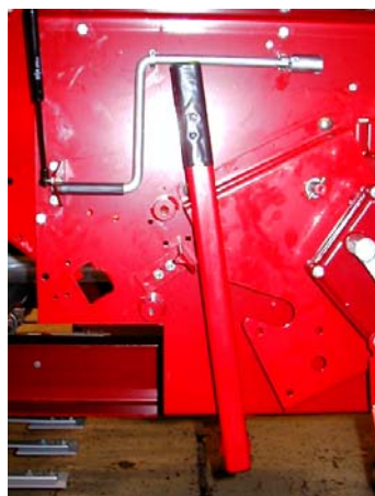
Lever to set the loading ramps for test or seeding.
