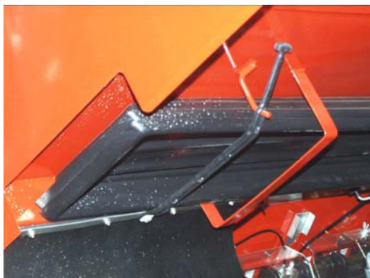
Test troughs locked with rubber strap when the machine is in normal seeding position.
