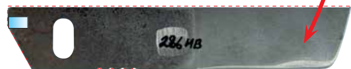
High-strength steel (S650) after the test
