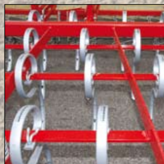
Four rows of tines for intensive soil preparation.
