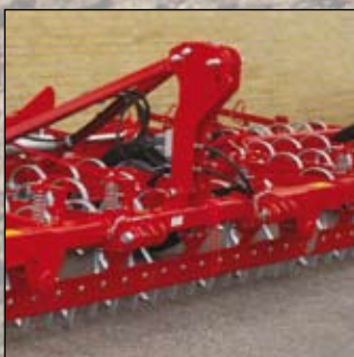
Standard for cat 2 or 3 mounting on tractor.
