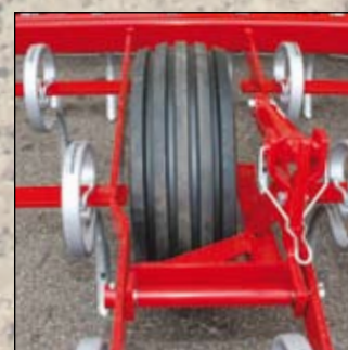
4 large rubber wheels for depth control – 24x8,00-14,5
