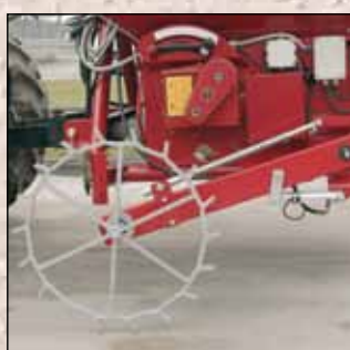
The application rates are controlled mechanical by a land wheel, as show, or electronical.
