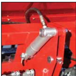
Hydraulic coulters pressure adjusting for NCS 3100 (optional).
