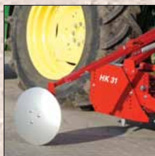
Hydraulic marker to vertical is standard.
