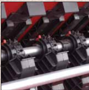
Combi seed wheels for large and small seeds.
