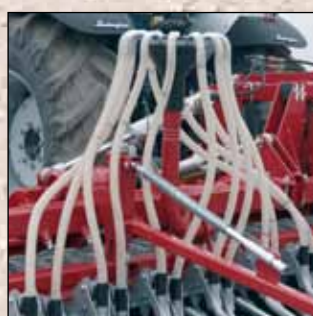
Even length of seed tubes is ensuring high accuracy of drilling.
