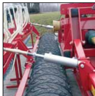
Hydraulic lift of coulters section for NCS 4100-5100 (optional).
