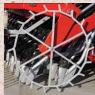
The large diameter land wheel ensures a constant speed drive in all conditions.
