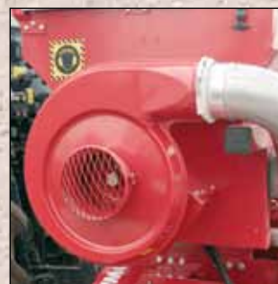
PTO or hydraulic driven blower for transporting of seed.
