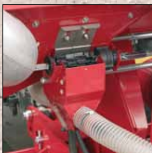
Metering unit with cell wheels.
