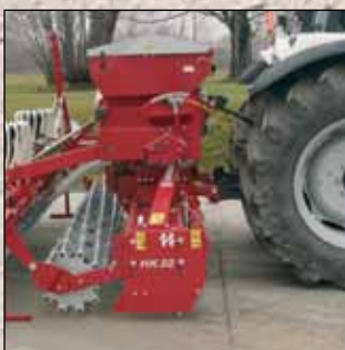
The large capacity seed hopper is mounted low and close to the tractor.
