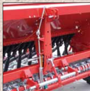
The coulters pressure is adjusted centrally by a spindle.
