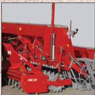
The weight of the drill is carried on the packer roller of the cultivator. The depth of drilling is adjusted in relation to the roller.
