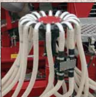
Distribution head with valve for tramlining.
