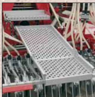
The sturdy loading platform makes filling of the seed hopper easier.
