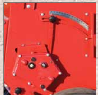
Stepless adjusting of application rate with Vario-K gearbox.
