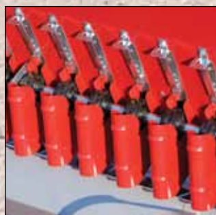
Precise metering system with peg-wheels.
