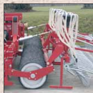
The mounting of the coulter section on the packer roller ensures an precise depth of drilling.
