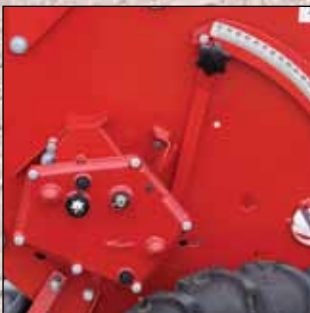
Steeple adjusting of application rate with Vario-K gearbox.
