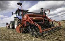
Heavy duty hydraulic combi hitch with MASTERLINE seed drill.
