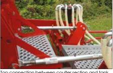
Top connection between coulter section and tank with adjustable top link, allowing level adjustment of coulter module,
