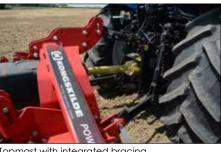
Topmast with integrated bracing.
