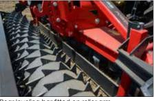
Rear leveling bar fitted on roller arm.
