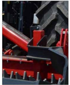
Height adjustment by spindle and suspended on rubber bumper.
