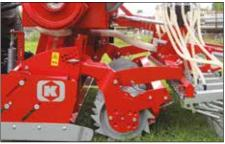
Parallelogram geometry of coulter section coupling. It is not necessary to adjust coulter section position when changing working depth.
