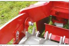
Quick coupling of coulter module on rear roller
