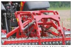
Heavy duty hydraulic combi hitch 3.5 tons lifting capaity.
