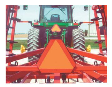
IMPORTANT NOTE: This unit has a narrow transport width and a high center of gravity which may pose a tipping hazard when folded for transport.
