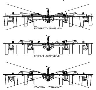
4. Once the machine is level front to back and side to side it's time to set the working depth. Turn the crank "1" clockwise to raise the machine or decrease working depth. Turn the crank counter clockwise to lower the machine or increase working depth. One full turn of the handle will change the depth approximately 3/16".
