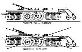
3. With the machine unfolded and in the raised position adjust the wings so they are level with the center. Adjust jamnuts "1" to position the cylinder anchor "2" so that the wing frames are level with the center frame. Move the cylinder eye forward to raise the wing and toward the rear to lower the wing. When the wingframes and center are level horizontally retighten the jamnuts "1". Note: It may be necessary to lower the machine for ease of adjustment.
