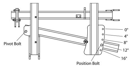
2. With the machine hooked to the tractor unfold and lower the machine so the coulter blades are 2" - 3" off the ground.
