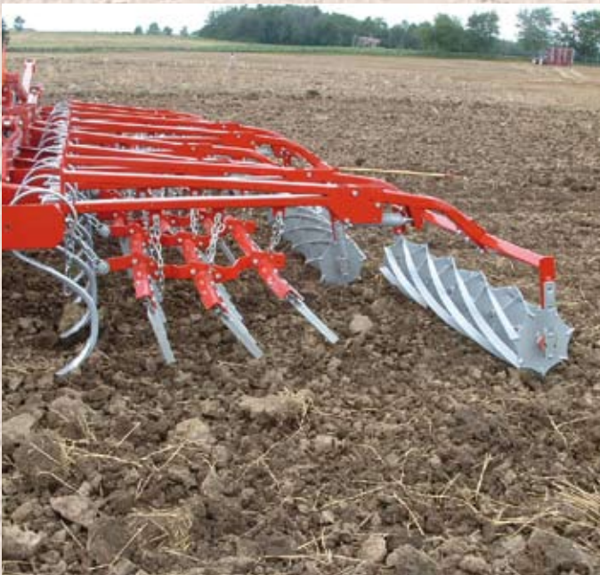
3 Spike Bar Unit with Single Row of Rolling Harrow.
