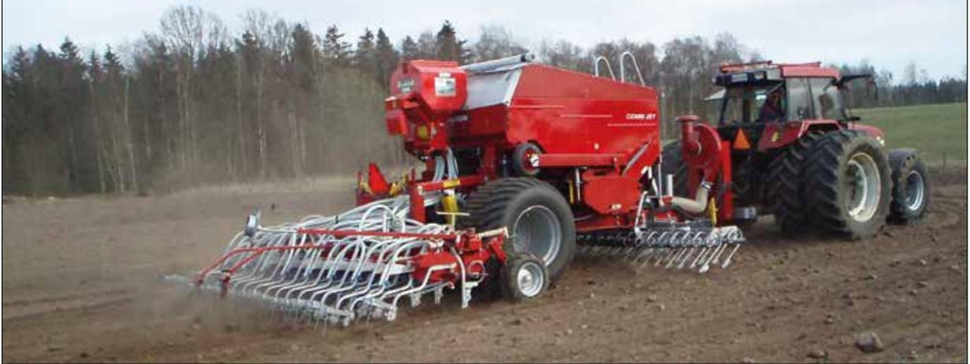
*Combi Jet 4504 is built on well proven principals for best possible seed placement. The strong coulters assembly with good clearance together with the possibility to mount the Multi Flex system and full width tyre packers in front of the coulters, give the option to cultivate, reconfirm, fertilise and seed in the same go. The machine above is equipped with optional grass seed box for simultaneous shallow grass establishment.*
