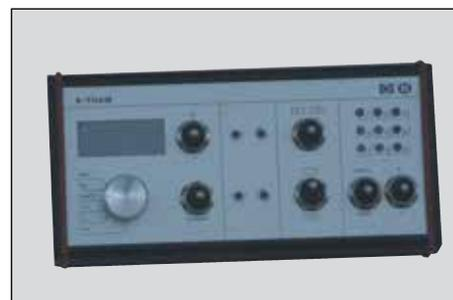
*Area counters, hopper level- and rotation controls and tramlining is managed by the K-Tram system*
