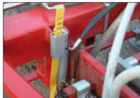
*Hydraulic coulter pressure adjustment cylinder with indicator placed on the outer end of the wing section.*
