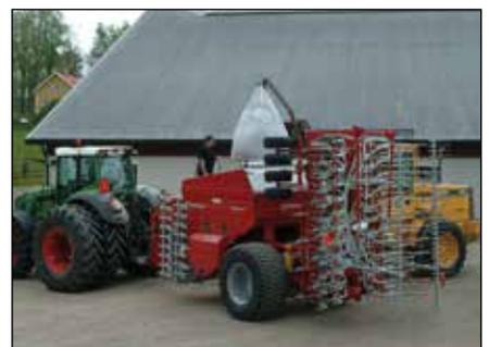
*The spring loaded roll-tarpaulin and the large hopper openings makes refilling quick and easy.*
