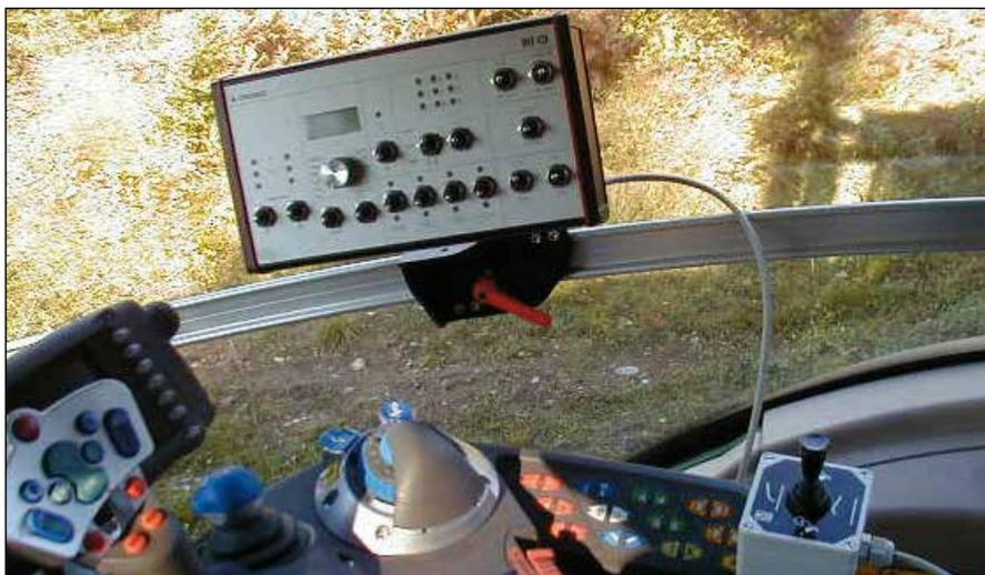
*K-Tronic offers possibilities to control application rates from the driver's seat while on the go.*
