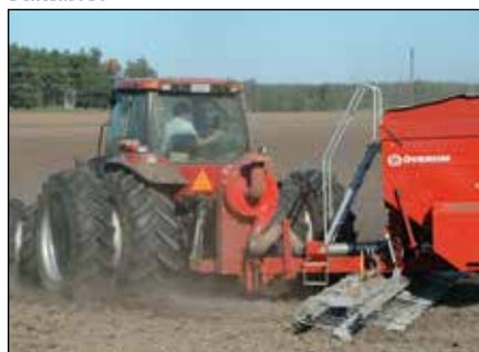
*The new cross shaft hitch makes the machine reach the corners and follows the tractor better when turning on the headland.*
