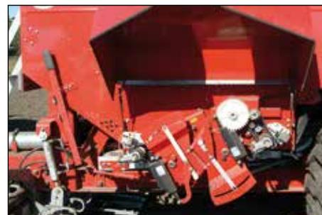
*Vario-K gearboxes controlled by K-Tronic offer possibilities to control the application rates while on the go.*
