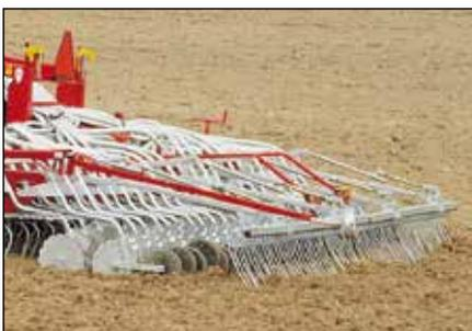
The individually spring loaded scalloped disc coulters on Multi Jet Disc have a pressure wheel consolidating over the seed row. A heavy rear harrow leaves an even loose surface.
