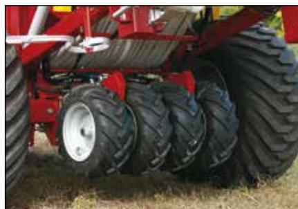
*Re-consolidation between the wheels of the tractor can be performed with an accumulator-loaded tyre packer between the large LGP-tyres.*
