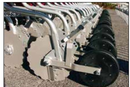
The depth control wheel is very easy and accurately set through a series of holes in steps of 5 mm.
