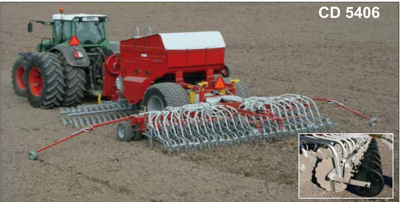
*Combi Jet 5406 equipped with Multi Flex system, Full width tyre packer, light following harrow and pre emergence marker, incorporates seedbed preparation, consolidation, fertiliser placement and seeding in one go. All Combi Jet models can also be delivered in disc coulters version for conditions with crop residues.*
