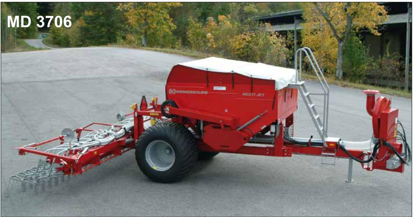
*Multi Jet 3706 base machine is a load carrying seed drill with low power demand. High drilling capacity can be achieved with a 100 hp tractor. Six metre working width and hopper capacity for more than 15 ha wheat gives high output.*
