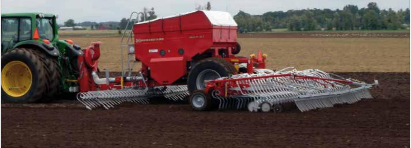
The Multi Jet 4608 Disc is developed to drill also in conditions with large amounts of crop residues. The spring loaded disc coulters are followed by a pressure wheel consolidating over the seed row, and at the same time keeping the maximum working depth of the coulters.
