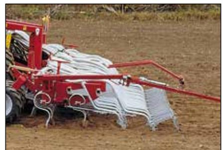
*The Multi Jet can be equipped with two rows of harrow tines in the coulter unit, placed to work the soil between each seed coulter.*
