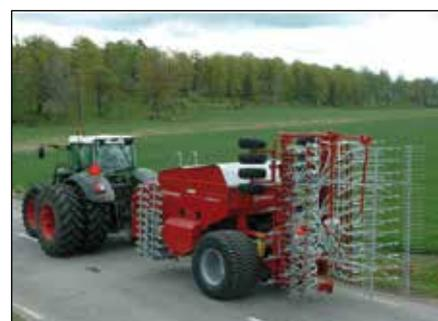
*All Jet-models from 4 to 8 m working width are hydraulically folded to 3 m transport width.*
