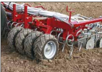
*Side packers with two, four or eight threaded rubber wheels can be mounted per side in order to achieve full width consolidation for 4, 6 and 8 m. working width.*
