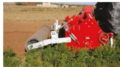
The sieve is spring loaded.
