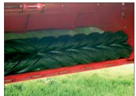
Roller conditioner: The roller conditioner is for more delicate crops that require a gentle conditioning in order not to lose the fodder value, e.g. alfalfa and clover.
