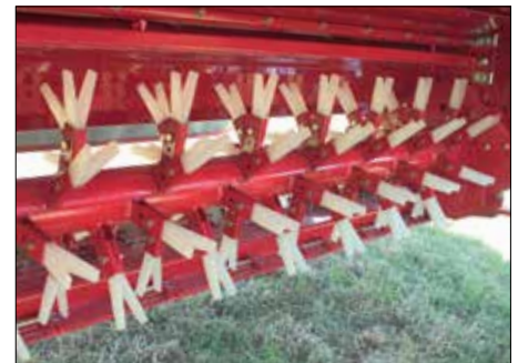
PE conditioner: PE-fingers provide a flexible and effective conditioning. The conditioner has a low static weight and requires minimum maintenance.
