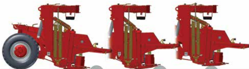
If the cutter bar hits a stone, the top spring is automatically compressed and the machine is lifted so that it can move undamaged over the obstacle.
