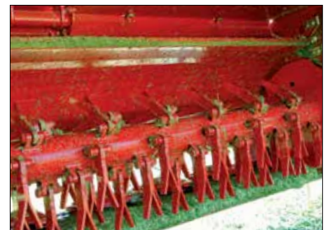
Flail conditioner: Steel flails can be used in areas with many large stones and extreme wear due to e.g. sand in the crop.
