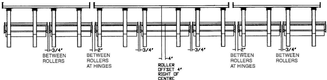
14. Mount left SS roller to the front or short hanger arms with the mounting plates and 1/2" x 3-1/2" bolts and locknuts provided. Be sure to butt the roller frames tight against the end of the hanger arms before tightening the locknuts. See diagram below.
