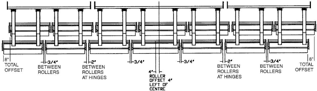
18. Continue mounting the rear rollers across the back of the cultivator until the assembly is completed. Remember to leave 3/4" between the end frames of the rollers and 2" between the centre section and wing rollers that meet at the hinges according to the diagram above.
