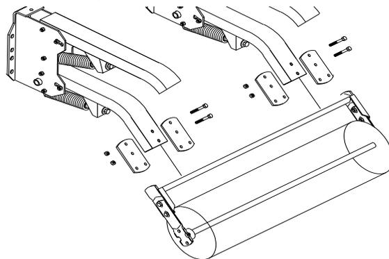
15. Mount the next front roller to the hanger arms in the same manner as in step 13 and 14. There should be 3/4" between the end frames of the rollers and 2" between the centre section and wing roller frames that meet at the hinges. See diagram previous page.
