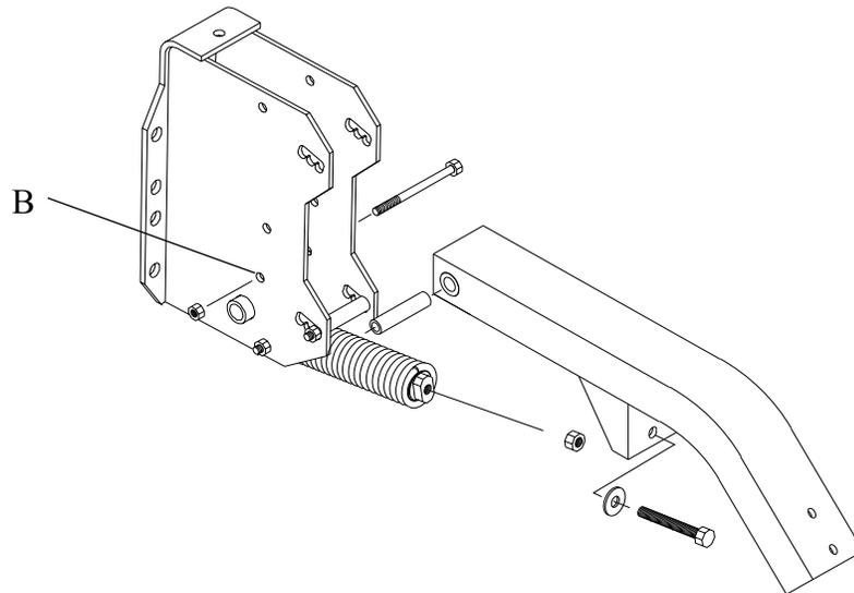
9. Install the upper spring assembly and upper (intermediate) arm in the same manner as steps 5 through 8. Use hole (C) for upper spring assembly and hole (D) for the upper hanger arms.
