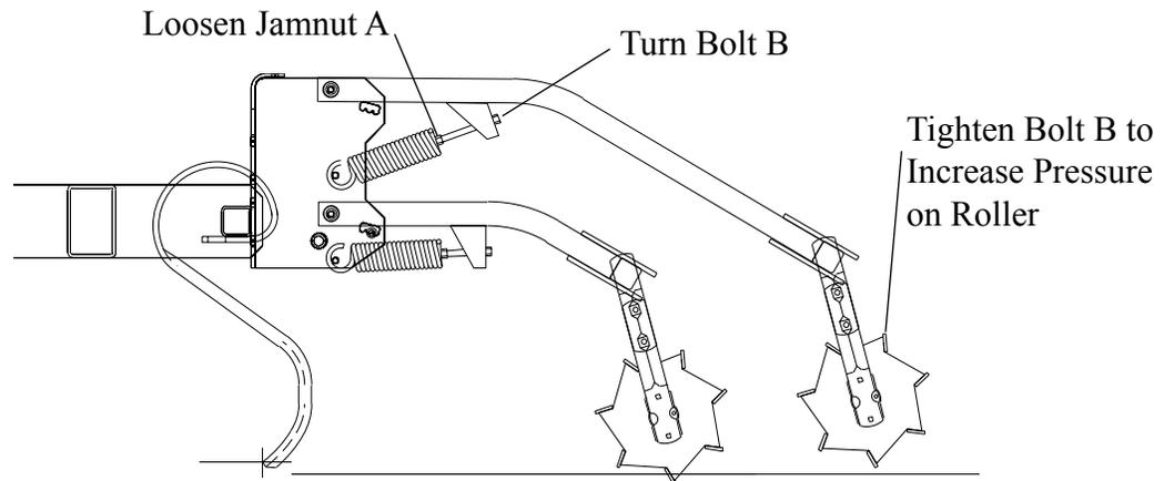
B) NOTE: In stony conditions the spring pressure should be reduced. Excessive pressure may cause damage to the rollers.
