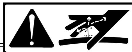
Check that the drawbar and the cutting unit can move freely before you activate the hydraulic cylinders. Make sure that no persons are near the machine when starting as there might be air in the hydraulic system which might lead to sudden movements.
