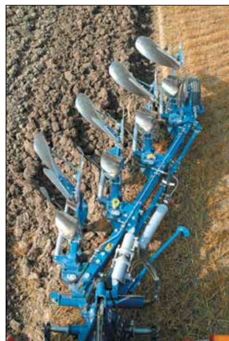
Precision drilling for the extensive bolt assembly has made it possible to use a heat-treated steel main frame tube.
