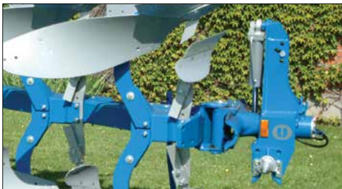
Xcelsior CX equipped with a new designed headstock which has a easy quick coupling of the cross.
