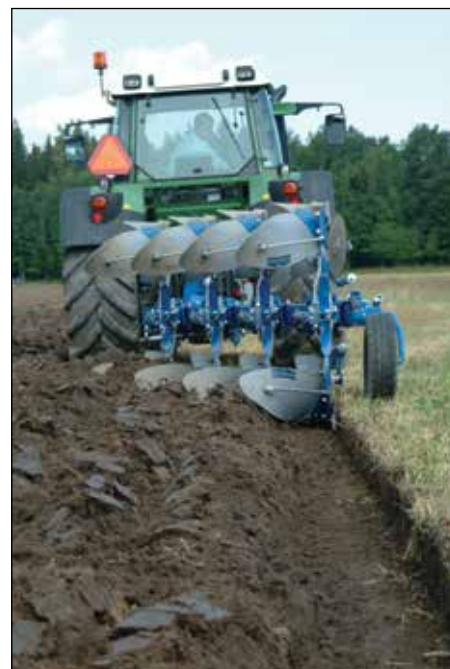
CX 4975 H, XL-bodies and EG-skimmers perform a well closed finish.
