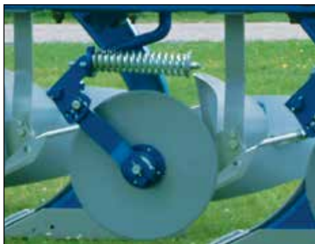
Spring loaded disc coulters. 18" or 20" plain or 20" rippled disc.
