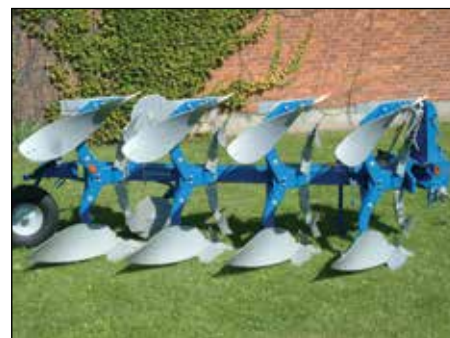
CX 4975 F with a new designed holder of the skimmers.
