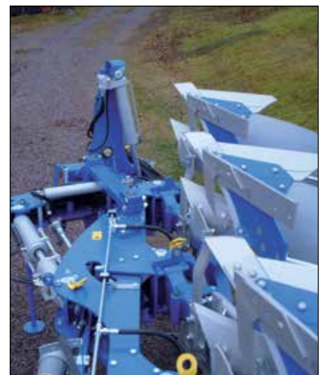
Beamhouses and double cylinder with long arms gives low stress and long lifetime. The furrow width is easy to adjust even in tough conditions.
