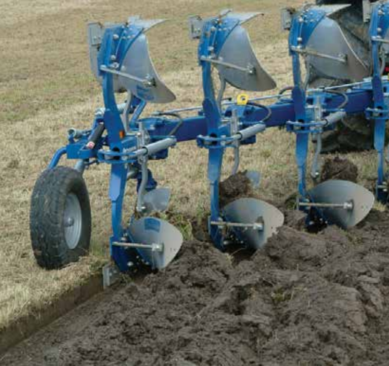
Shallow ploughing with a working depth of 11 cm
