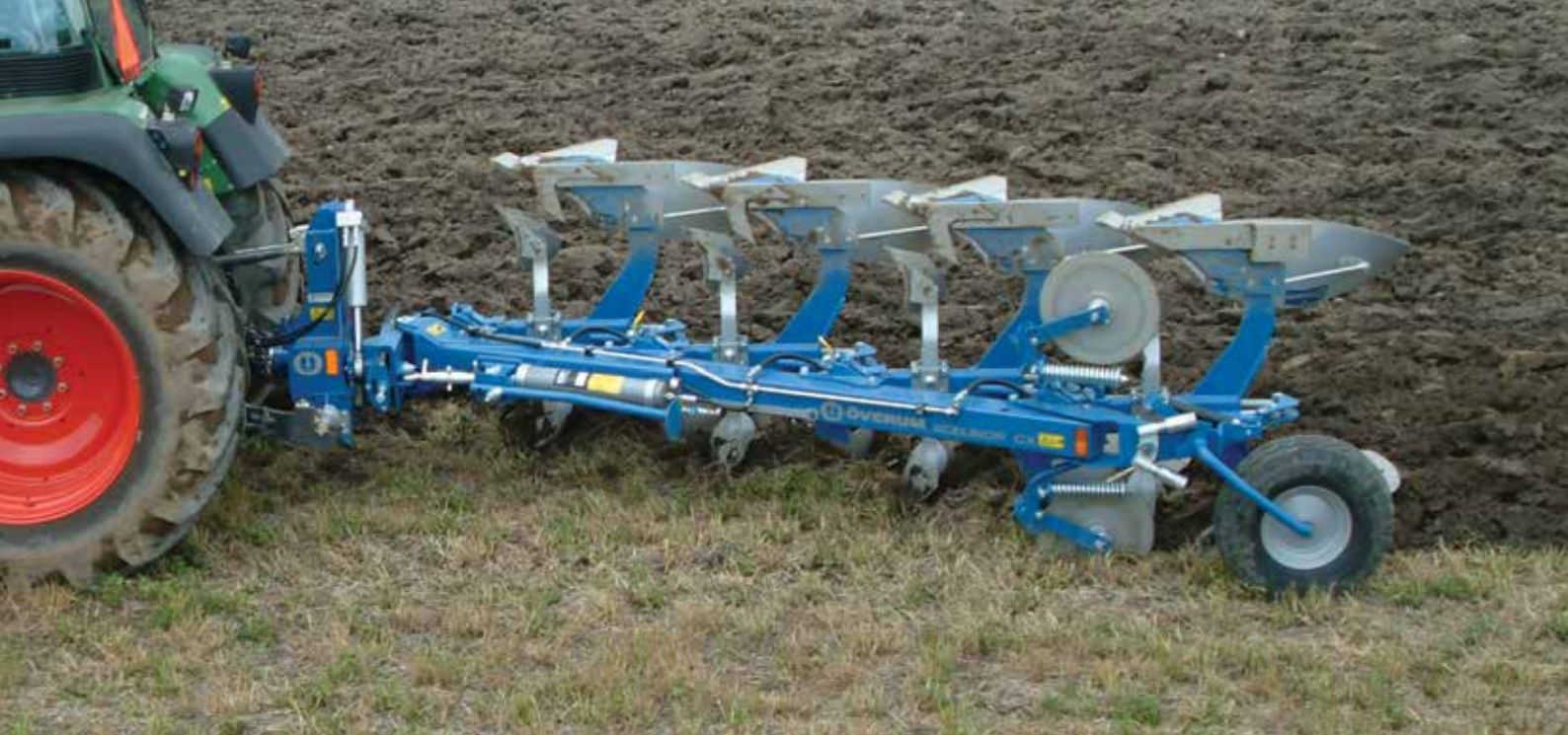
CX 4975 H with EG-skimmers. 90 cm point to point clearance makes room for effective skimming equipment.
