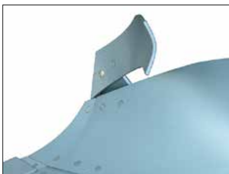
Trashboard. Good clearance for straw. Not recommended for sticky soils.
