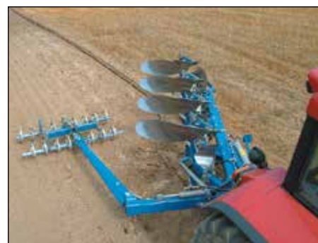
Nivell integrated furrow leveller from three to four furrows.
