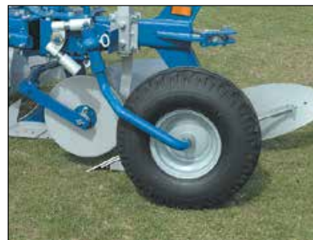
Combi wheel for depth control/transport 10.00 x 12. Diameter 710 mm, width 264 mm.
