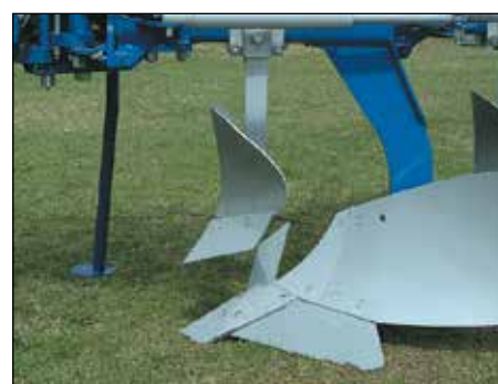
Skimmer EM. Handles large amounts of crop residues. Works best with fin coulters.
