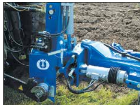
Heavy duty headstock with quick coupled cross shaft and alignment cylinder.
