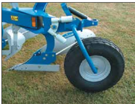
Depth wheel rubber 7.00 x 12. Diameter 645 mm, width 182 mm.
