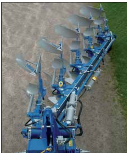
The favourable geometry in the regulation system makes it possible to adjust the working width on the go with relatively low pressure.
