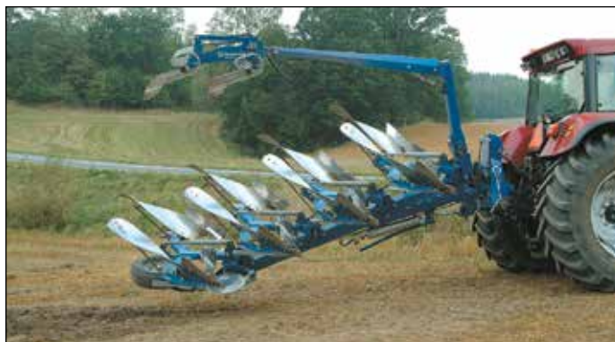
Bodies turning over the frame require slightly higher lift capacity. When the bodies are turning under the frame (see page 3) a lower lifting height is sufficient.
