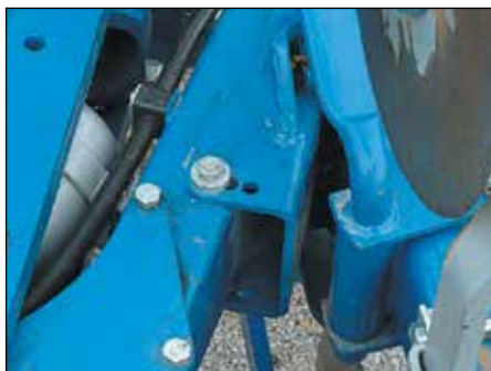
The furrow width can be adjusted in three steps.
