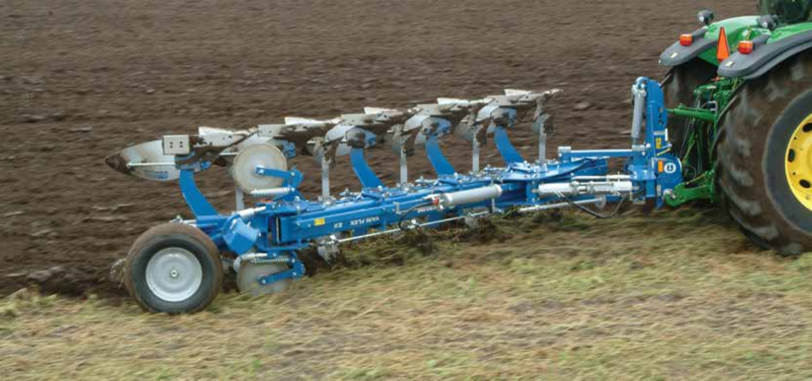
Vari Flex EX 5975 H is a heavy duty dimensioned plough, for tractors up to 300 hp.
