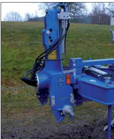
Heavy duty headstock Cat 3 with 150/180mm pivot shaft and needle roller bearings for an efficient distribution of high loads. Cross shaft with quick coupling and possibility to adjust in height and length. Butterfly transport lock as standard.
