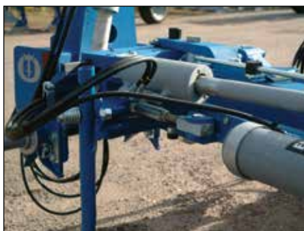
With the turnbuckle all side forces are balanced out for minimum draft requirement.
