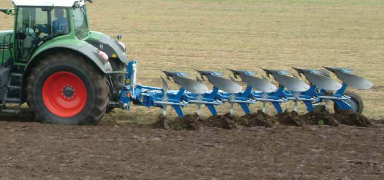
Vari Flex EX 6975 H with hydraulic adjustment of the furrow width up to 3.3 m.
