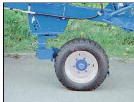
Combi wheel in forward position for Xcelsior DX models. Diameter 755 mm, width 275 mm.
