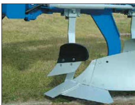
Skimmer EP. Plastic mouldboard for the best scouring properties.
