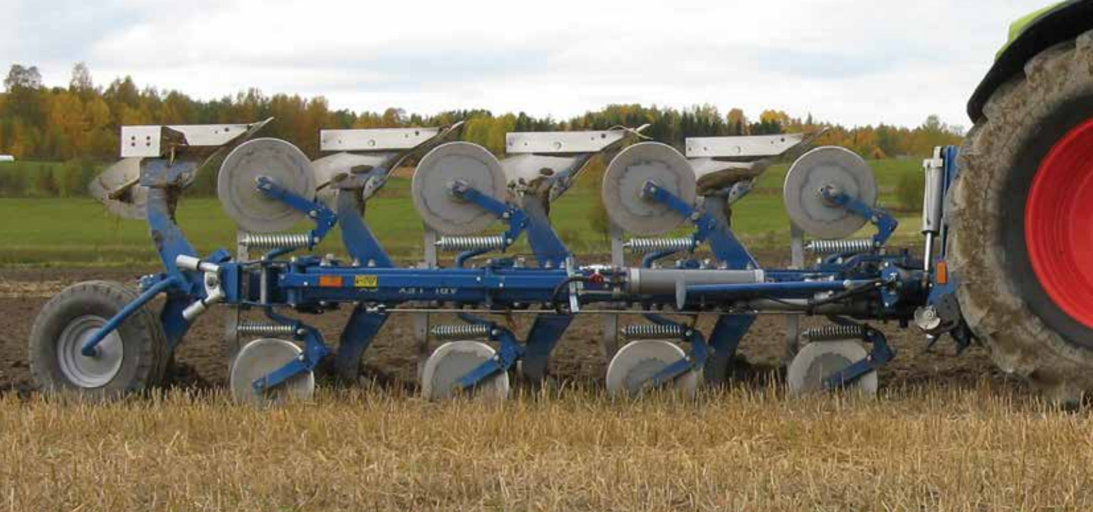
Vari Flex CX 4975 H with spring loaded disc coulter and EG-skimmers. Hydraulic furrow width adjustment from 12 to 20 inches.
