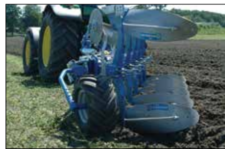
The new heavy duty depth wheel with extended adjustment range has a wide tyre with good carrying capacity. The turn over movement is effectively damped by an adjustable friction brake.
