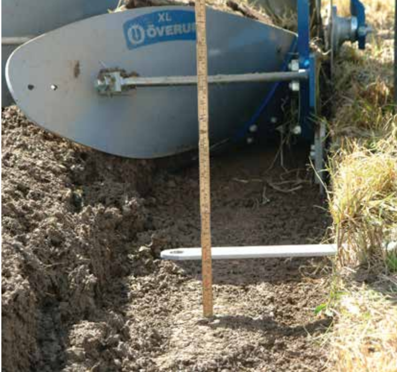
Shallow ploughing with a working depth of 11 cm
