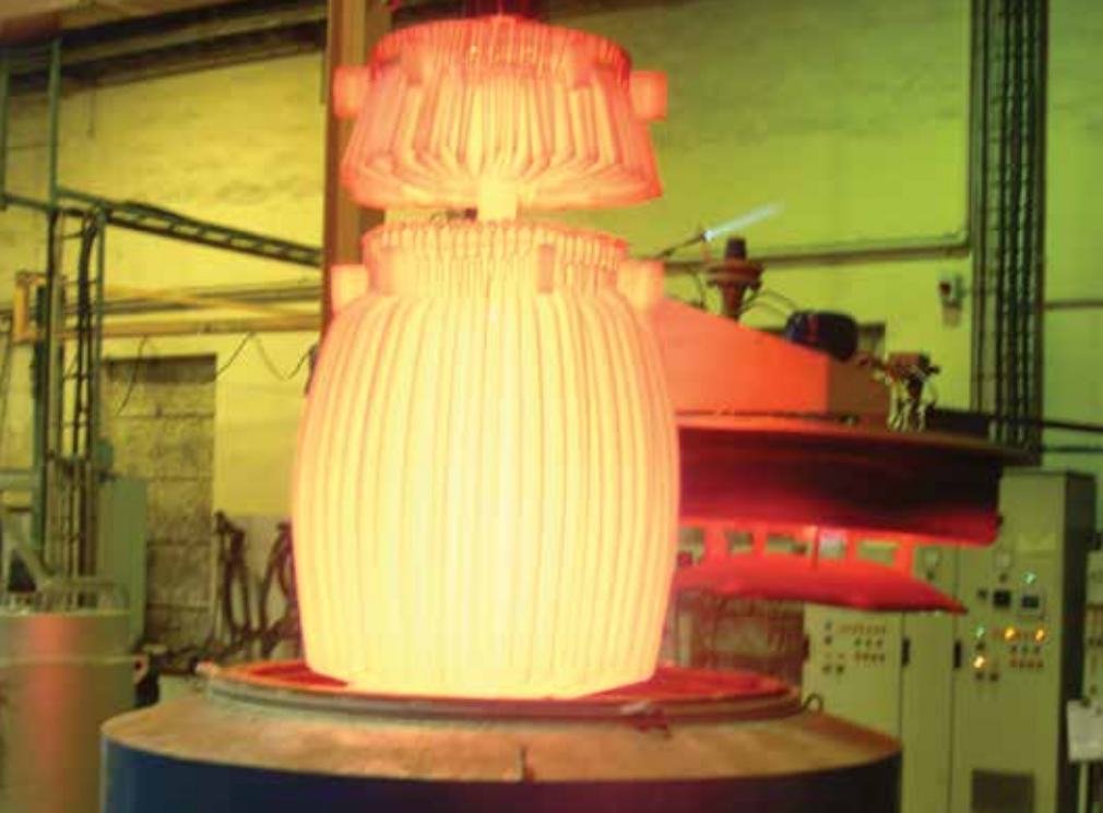
Carburizing of mouldboard blanks.
