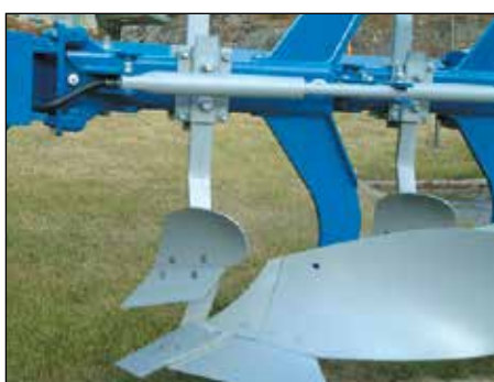
Skimmer EG. Wide shallow cut. Works well with both fin coulters and disc coulters.
