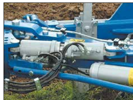
The double cylinder memorises the furrow width setting during the alignment and turnover action.
