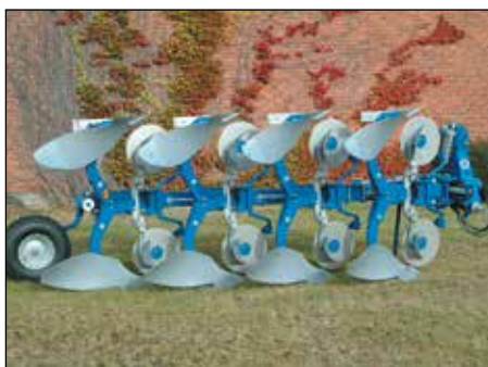
Vari Flex CX 4975 F with fixed disc coulters and EG skimmers. Bodies as well as skimmers have individual shear bolts.
