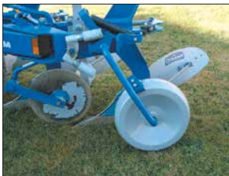
Depth wheel steel. Diameter 500 mm, width 160 mm.
