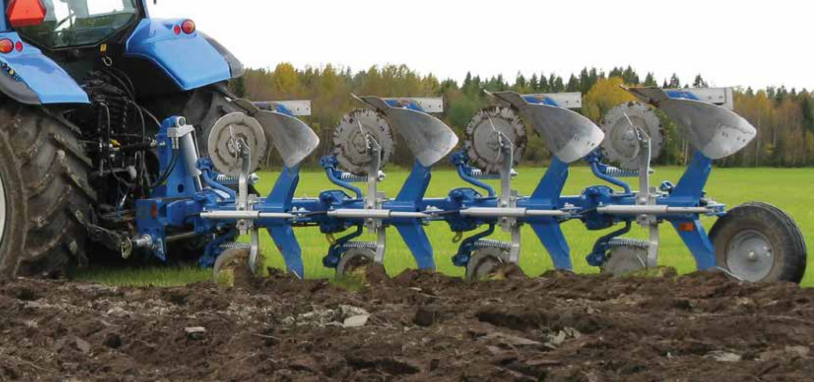
Xcelior CX 4975 H equipped with disc coulters and EG-skimmers. Working width adjustable between 140-180 cm.
