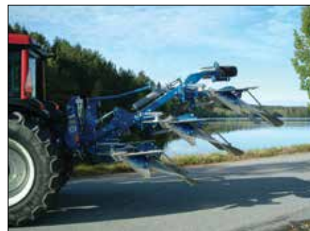
Due to the fact that the bodies are turning under the frame, the centre of gravity comes close to the tractor, and the plough becomes easy to lift.
