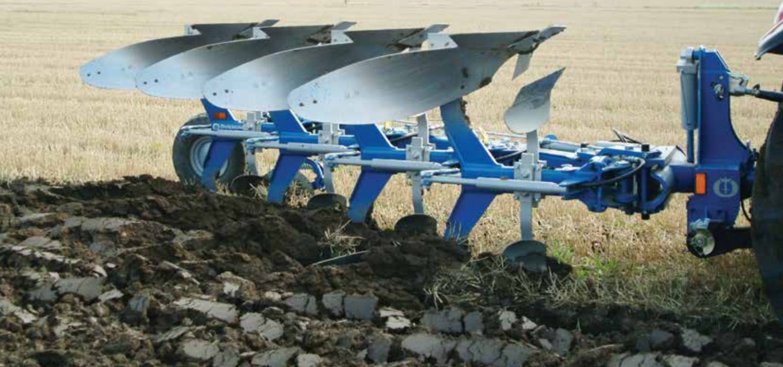
Vari Flex CX 4975 H with fin coulter and EG-skimmers. Hydraulic furrow width adjustment from 1.2 to 2 m.
