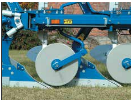
Fixed disc coulters. 18" or 20" plain or 20" rippled disc.
