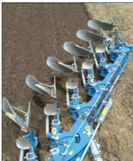
The pulling line can be adjusted precisely, which saves diesel and reduces the wearing. Strong main beam 220x120mm without welding. Depth transport wheel 260/70-16 optional 340/55-16.
