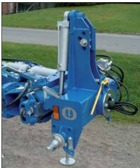
The heavy duty headstock with 150 mm pivot shaft and needle bearings is dimensioned for tractors up to 200 hp.
