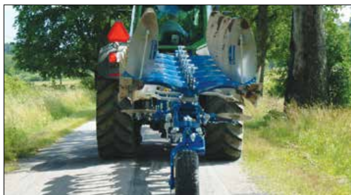
Switching to butterfly position unburdens the tractor during transport.
