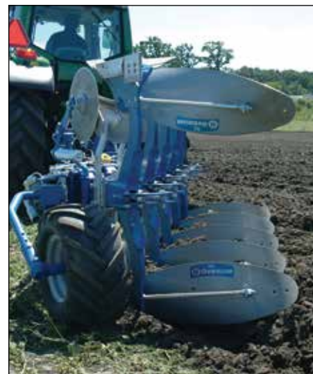
The new heavy duty depth wheel with extended adjustment range has a wide tyre with good carrying capacity. The turn over movement is effectively damped by an adjustable friction brake.
