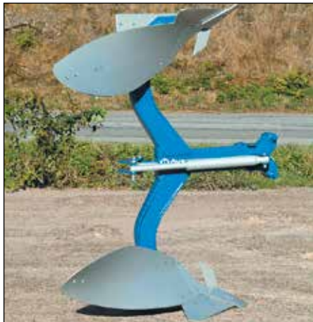
With high clearance profile beams large amounts of crop residues will flow through.
